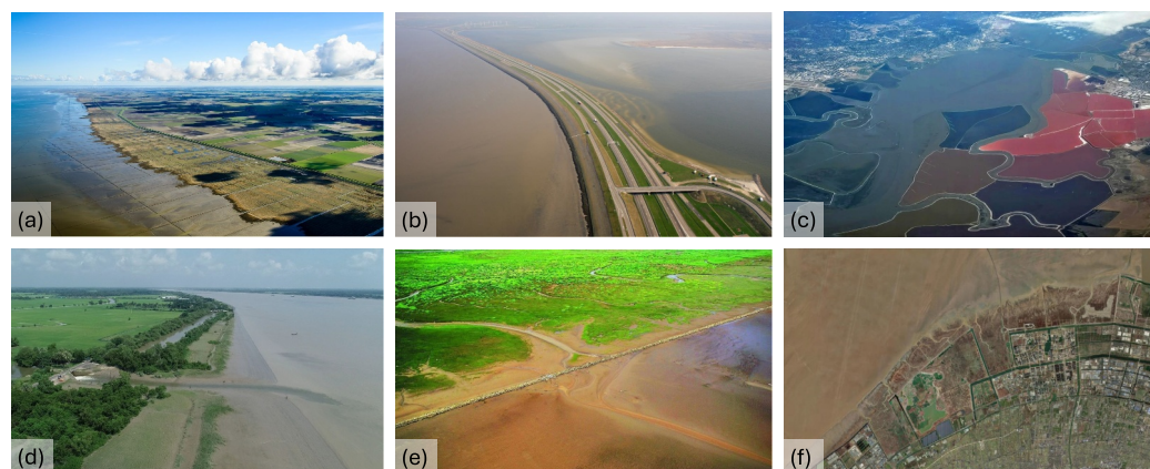
Figure 1. Visual overview of land reclamation types in type-dominated estuaries: a centuries-old land reclamation method gradually converting intertidal area to agricultural land (Dutch-German Wadden Sea, a); a dam closing off the largest land reclamation of the world (South Sea, b); Salt ponds (South San Francisco Bay, c); a polder with former creek now functioning as drainage channel (Bangladesh, d); recent concrete embankments preparing wetlands for reclamation (Yangtze River mouth, e); and gradual conversion from salt marsh to urban area (Hangzhou Bay, f). Photos courtesy of Siebe Swart (a), Staartjes Fotografie Deventer (b), https://commons.wikimedia.org/wiki/File:South_San_Francisco_Bay_salt_ponds_and_wildlife_refuges.jpg (c), https://www.bluegoldwiki.com/index.php?curid=2281 (d), SKLEC (e), and https://map.tianditu.gov.cn (f).
