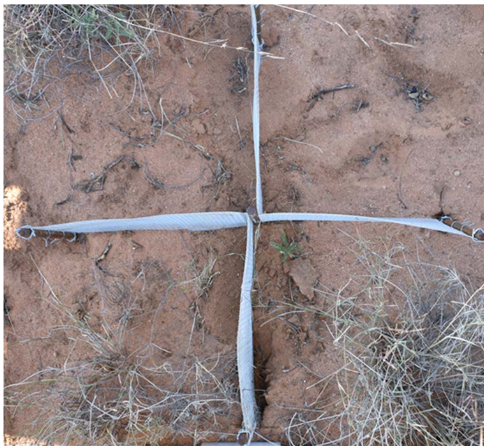
FIGURE 6-7 A connectivity modifier (ConMod) stabilizing sand at the U.S. Department of Agriculture–Agricultural Research Service (USDA-ARS) Jornada Experimental Range. SOURCE: Photo courtesy of Michael Fischella.
