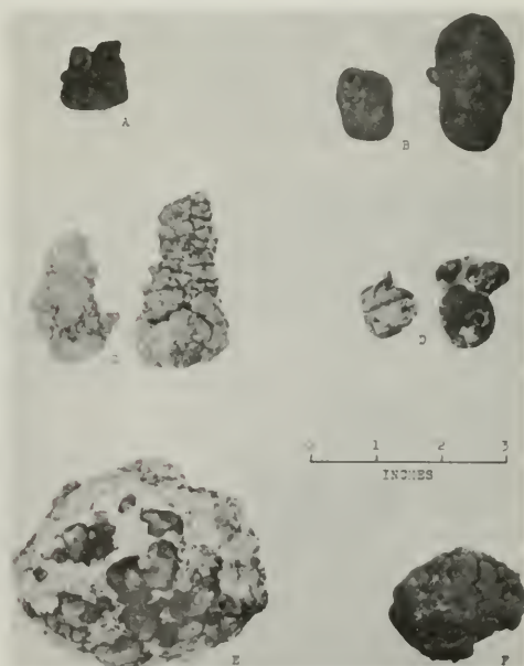
Photo 4. Manganese nodules from the north Pacific, illustrating a few of the many shapes they assume in their growth process. The location data for the individual nodules are: A.) N. 29° 58', W. 125° 55', depth 4,325 m.; B.) N. 23° 17', W. 138° 15', depth 4,890 m.; C.) N. 22° 30', W. 113° 08', depth 3,600 m.; D.) N. 14° 11', W. 161° 08', depth 5,652 m.; E.) N. 9° 57', W. 137° 47', depth 4,930 m.; F.) N. 21° 27', W. 126° 43', depth 4,300 m.
