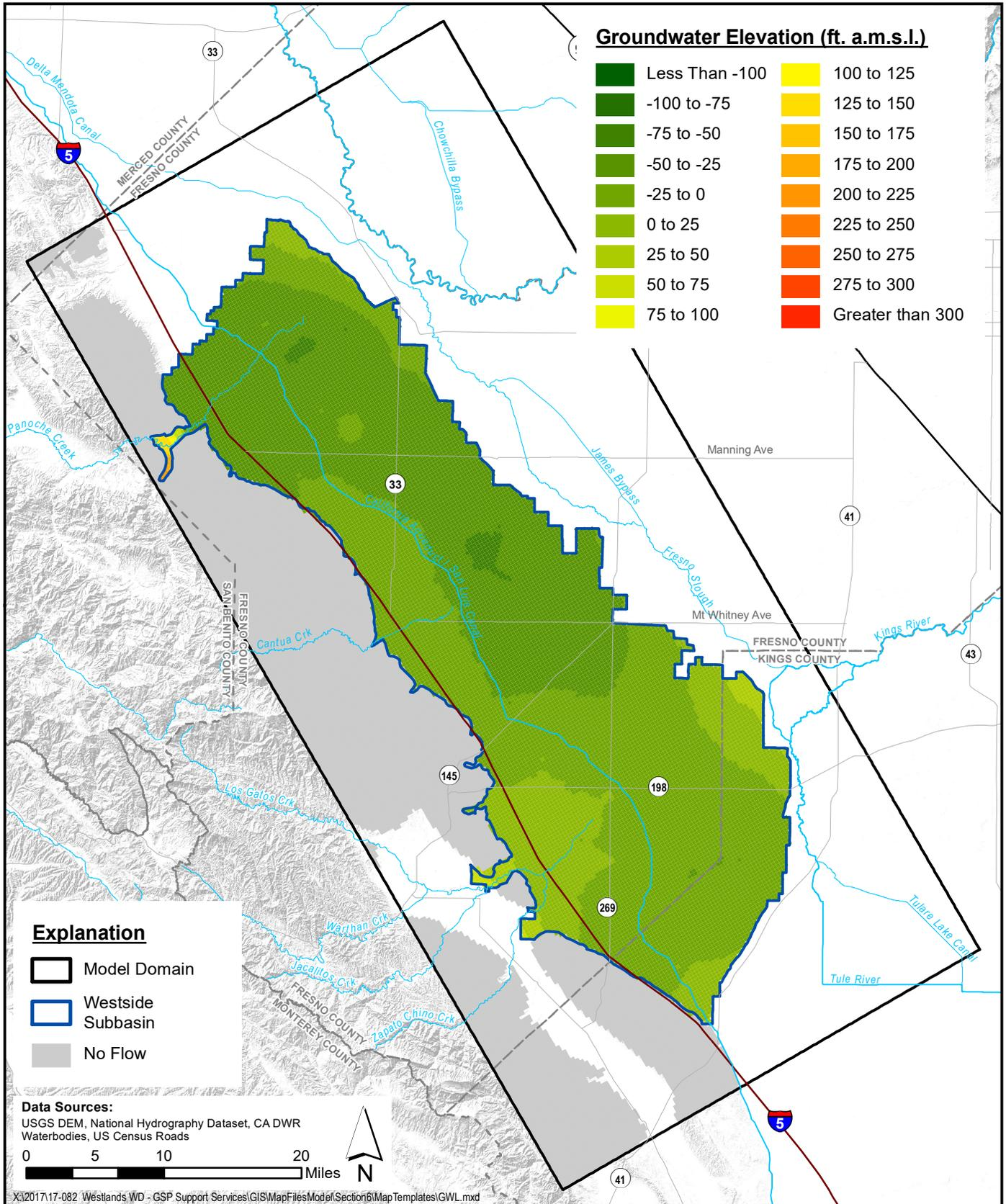
**Simulated Groundwater Elevation - Lower Aquifer
