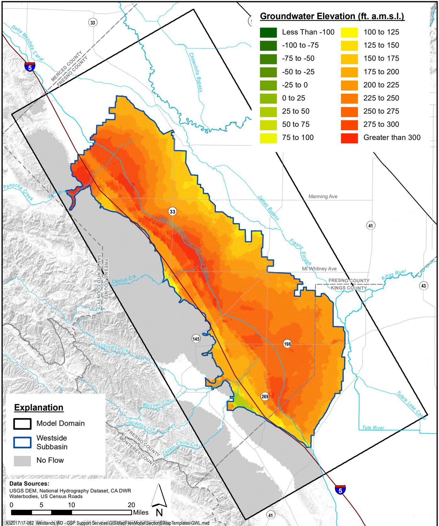
**Simulated Groundwater Elevation - Shallow Zone
