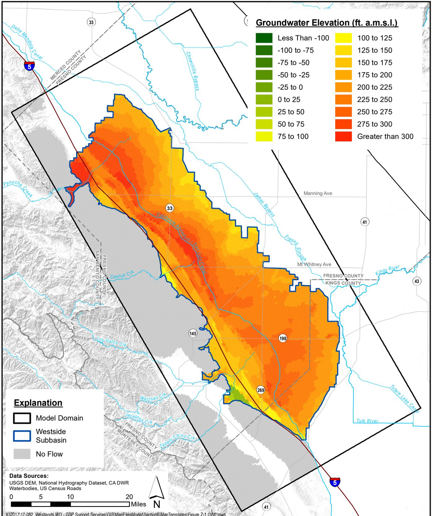
**Simulated Groundwater Elevation - Shallow Zone
