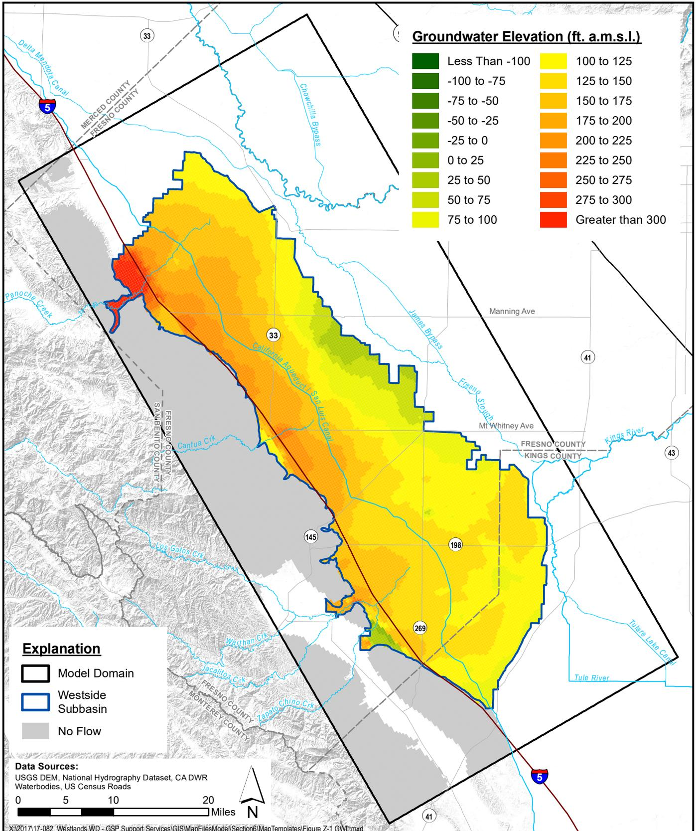
**Simulated Groundwater Elevation - Upper Aquifer
