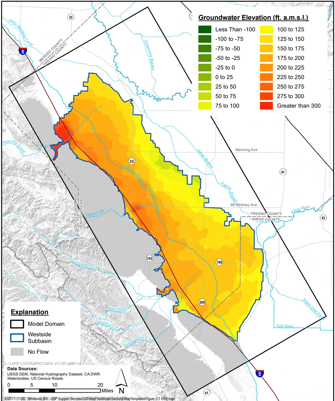
**Simulated Groundwater Elevation - Upper Aquifer
