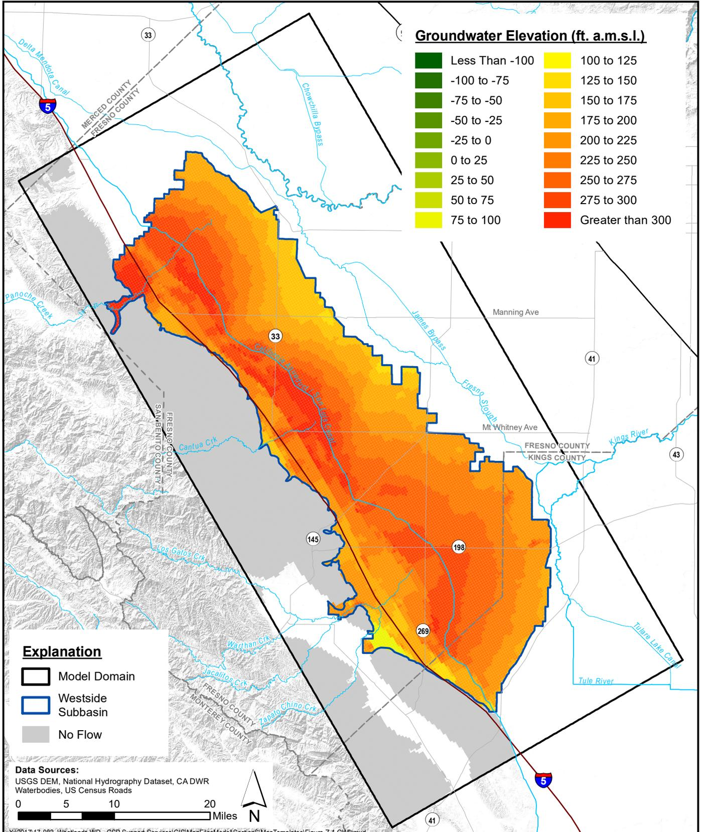
**Simulated Groundwater Elevation - Shallow Zone
