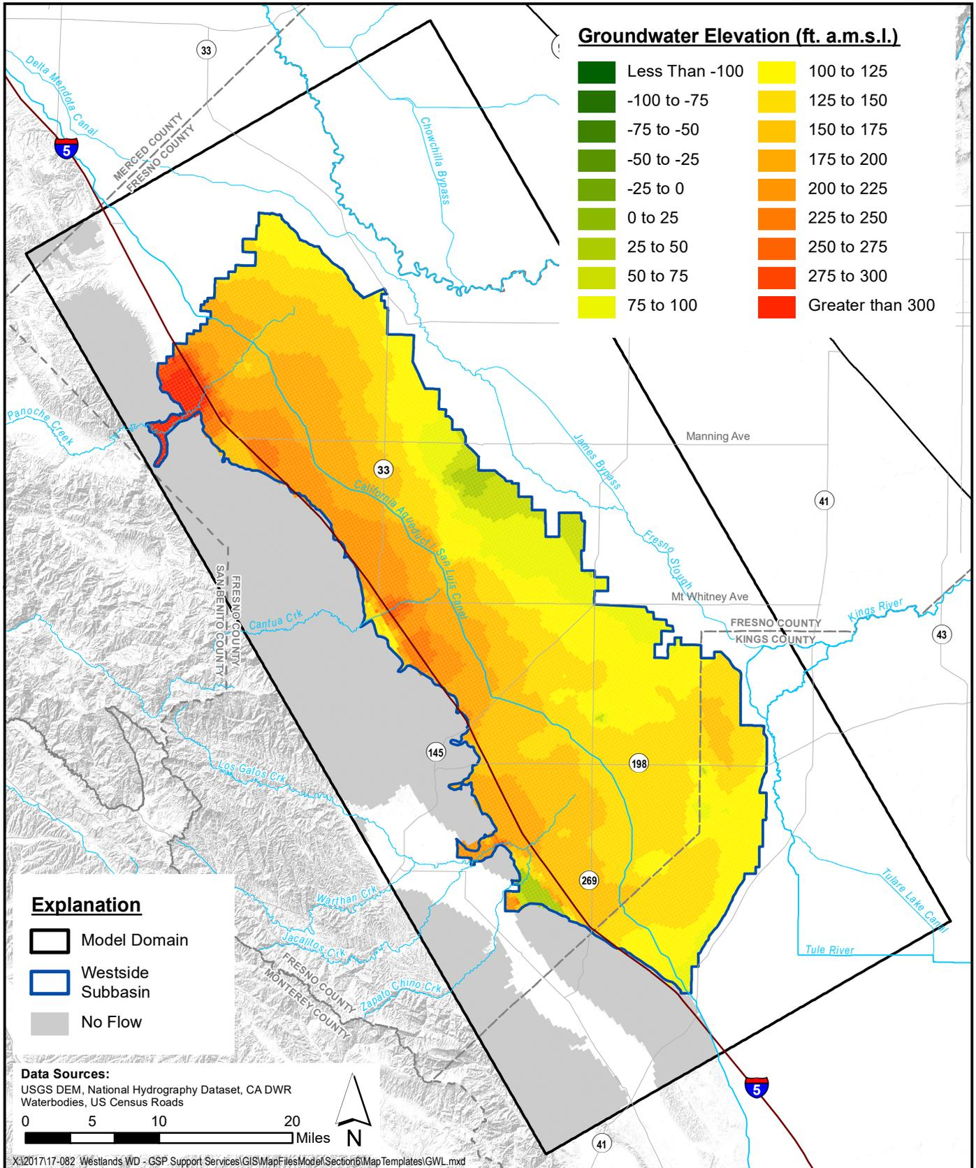
**Simulated Groundwater Elevation - Upper Aquifer
