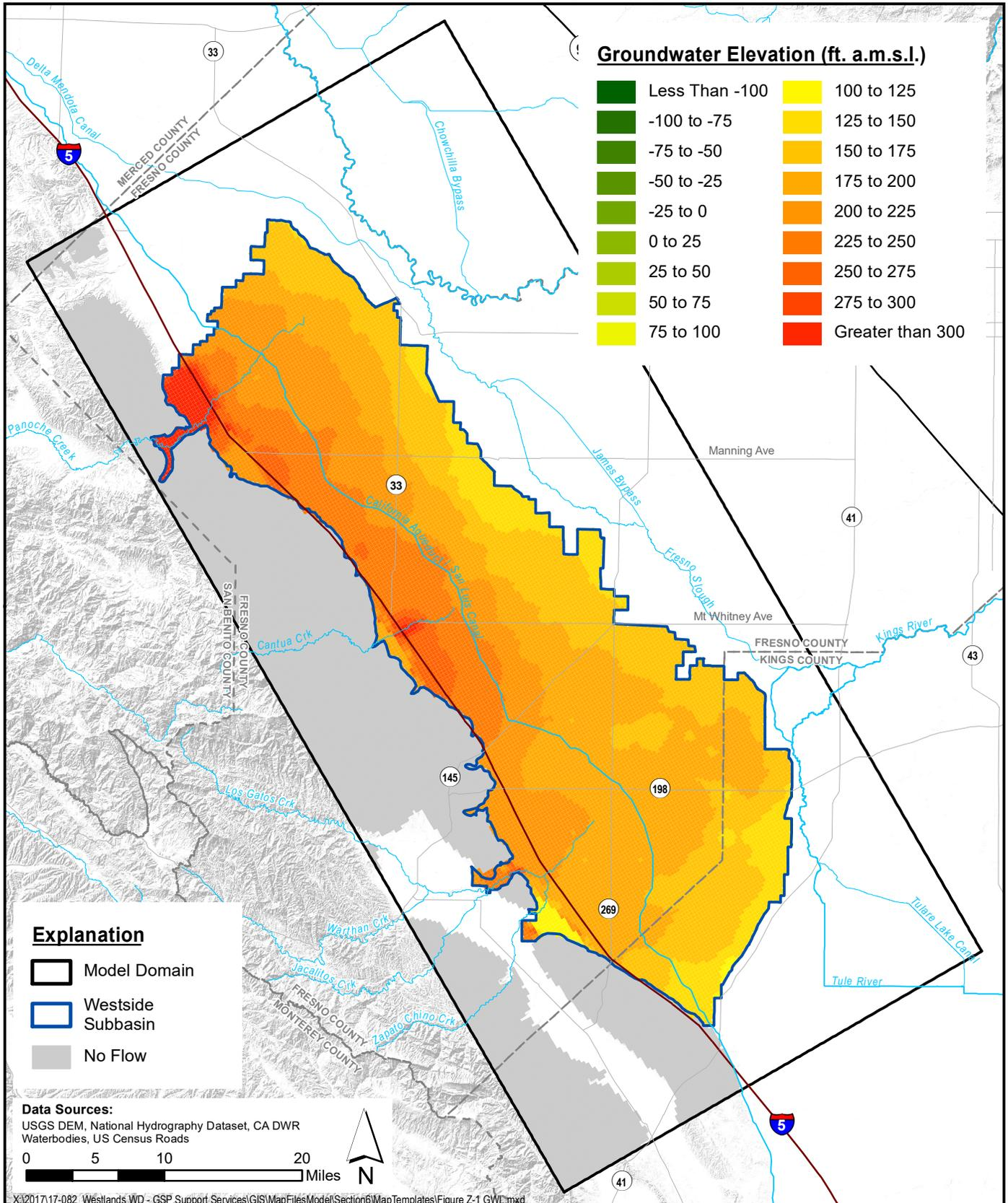
**Simulated Groundwater Elevation - Upper Aquifer
