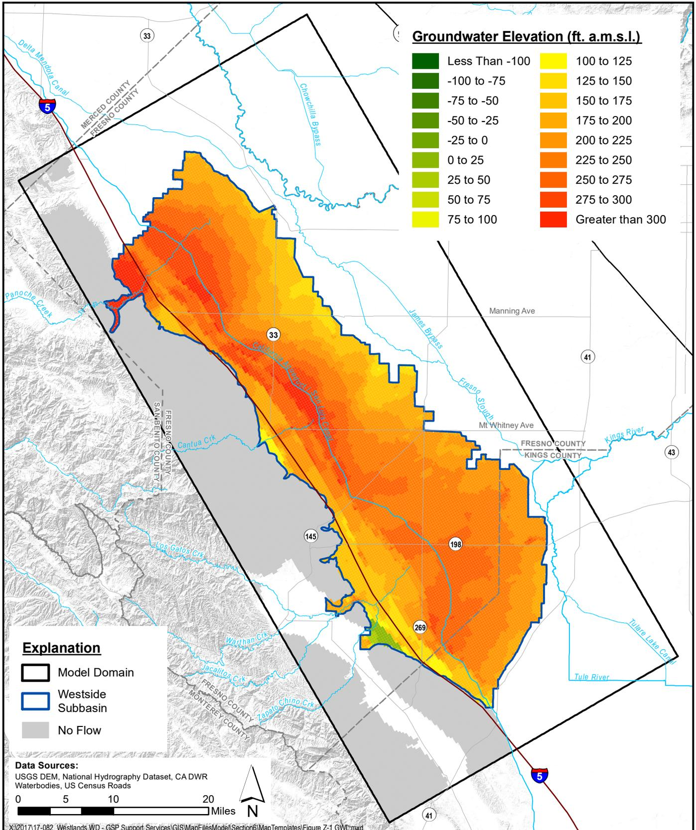
**Simulated Groundwater Elevation - Shallow Zone
