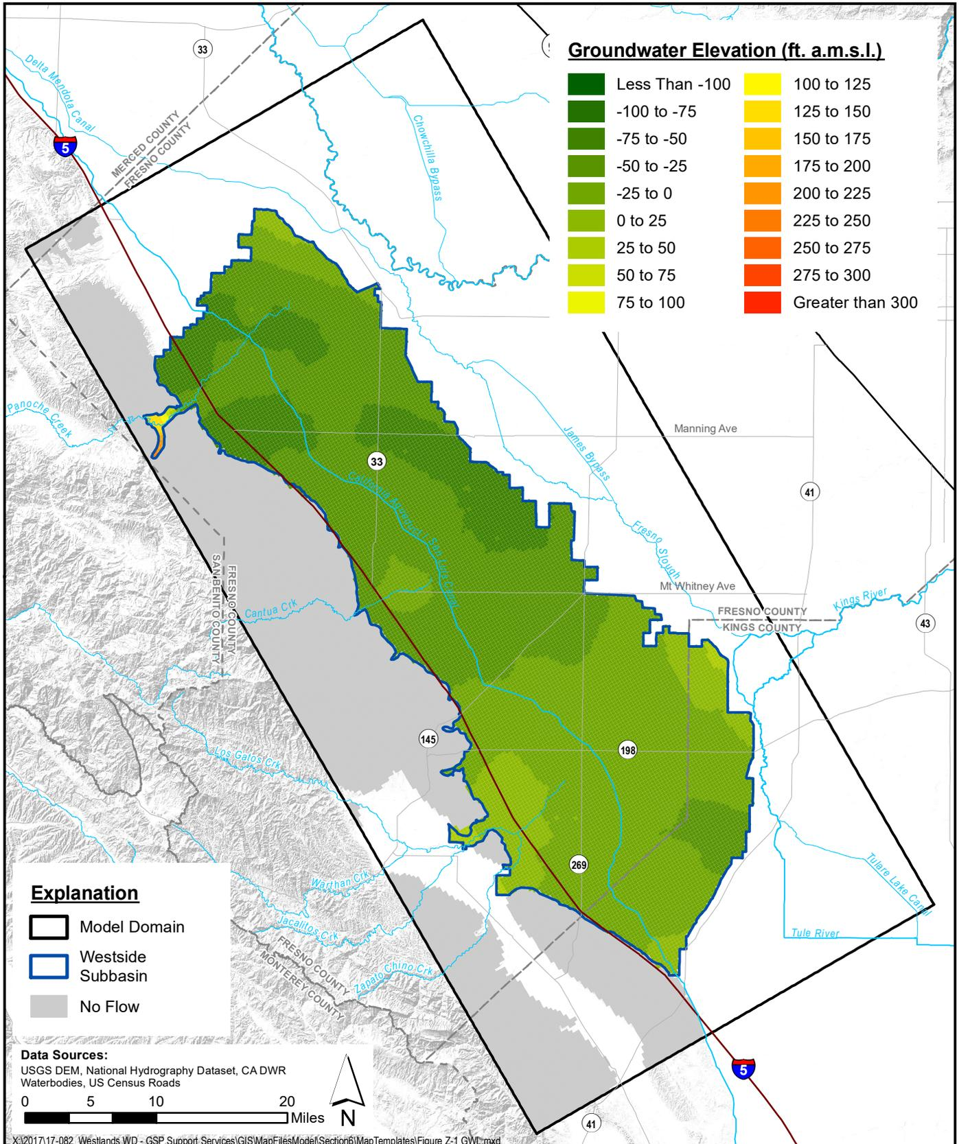
**Simulated Groundwater Elevation - Lower Aquifer
