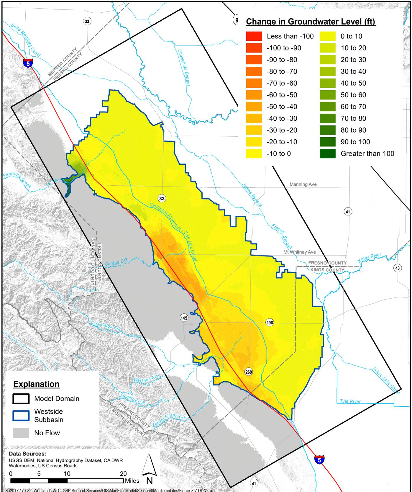
**Simulated Change in Groundwater Elevation - Shallow Zone
