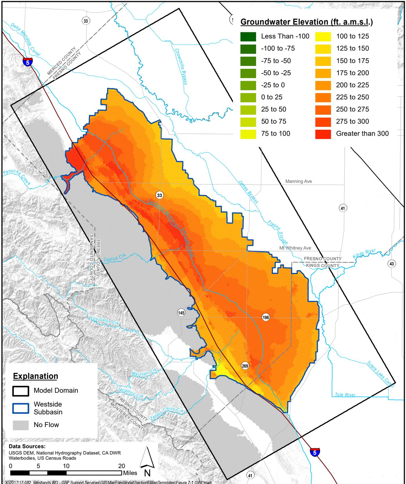
**Simulated Groundwater Elevation - Shallow Zone
