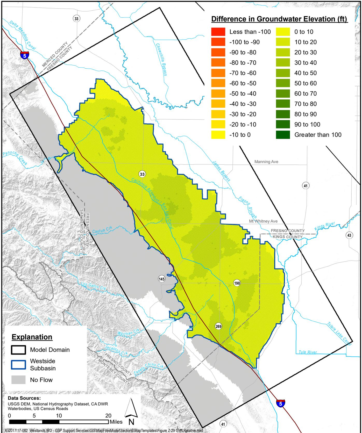
**Project Impacts on Groundwater Elevation - Lower Aquifer
