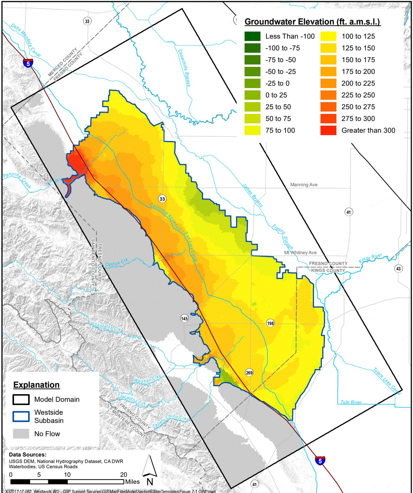
**Simulated Groundwater Elevation - Upper Aquifer
