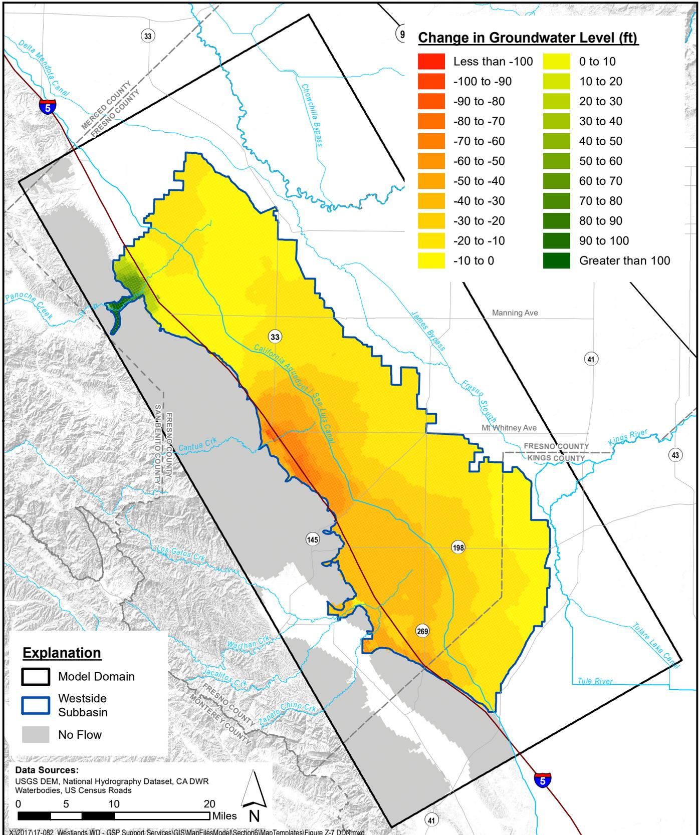
**Simulated Change in Groundwater Elevation - Upper Aquifer
