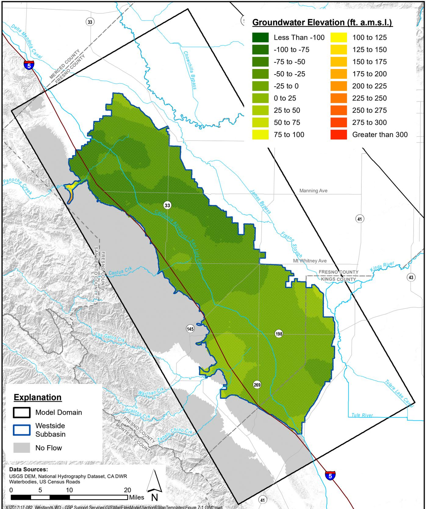
**Simulated Groundwater Elevation - Lower Aquifer
