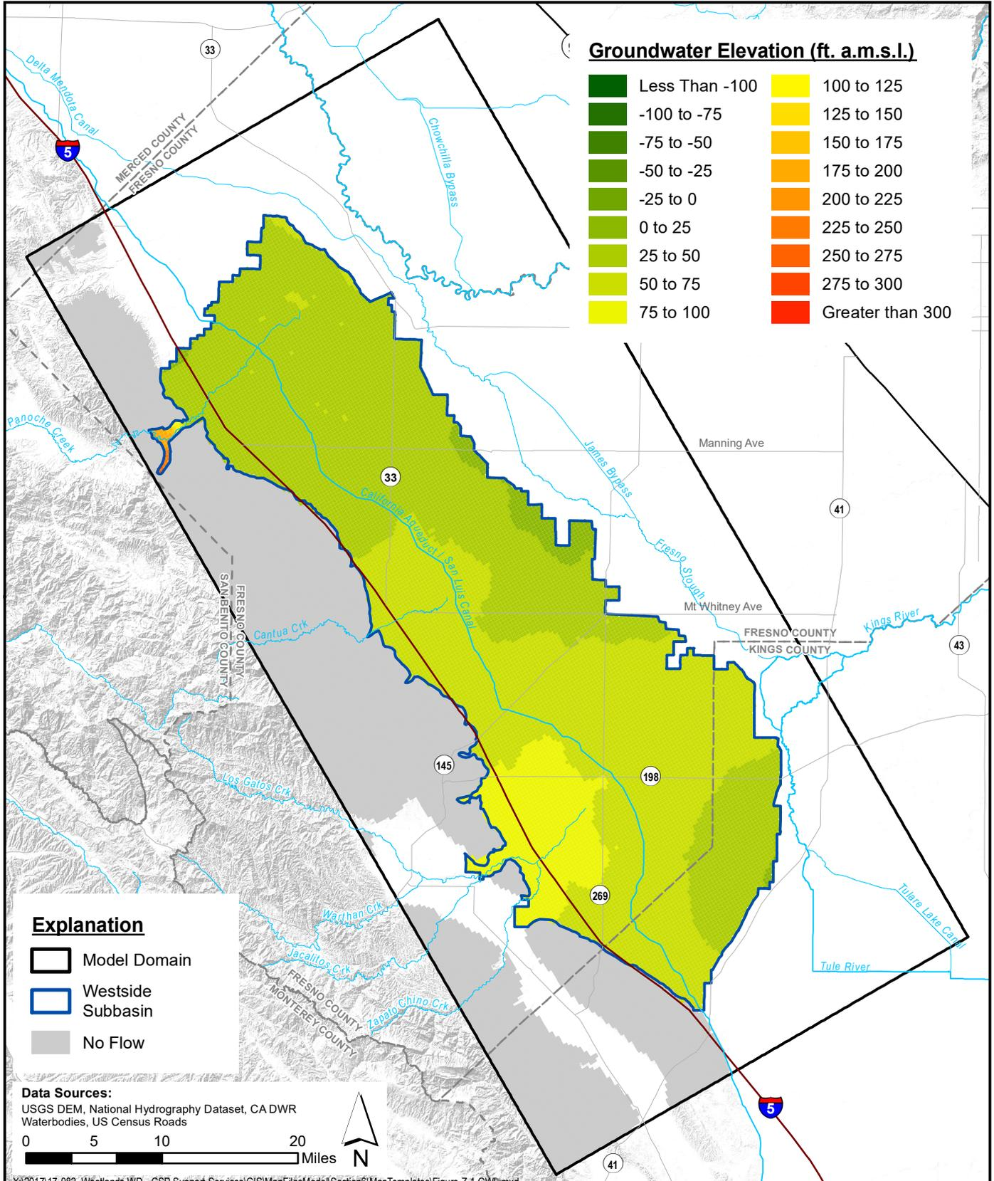
**Simulated Groundwater Elevation - Lower Aquifer
