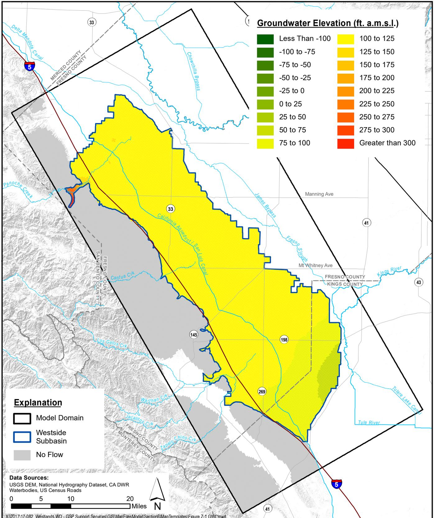
**Simulated Groundwater Elevation - Lower Aquifer
