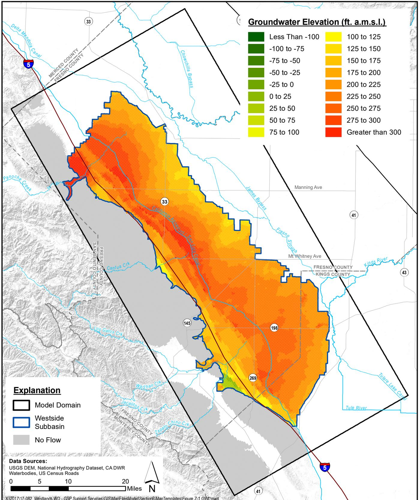
**Simulated Groundwater Elevation - Shallow Zone
