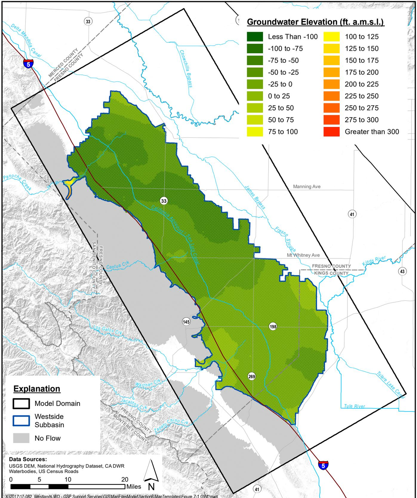
**Simulated Groundwater Elevation - Lower Aquifer
