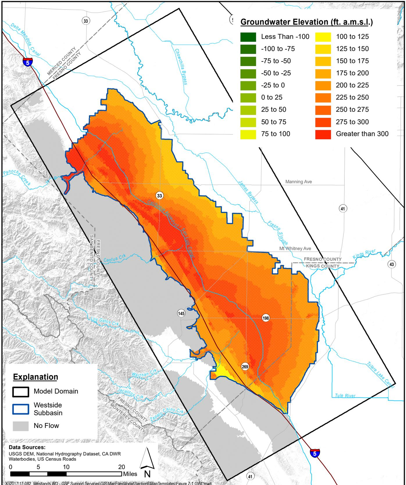
**Simulated Groundwater Elevation - Shallow Zone
