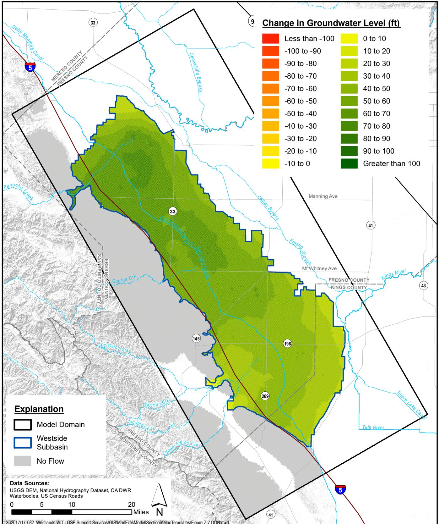
**Simulated Change in Groundwater Elevation - Lower Aquifer
