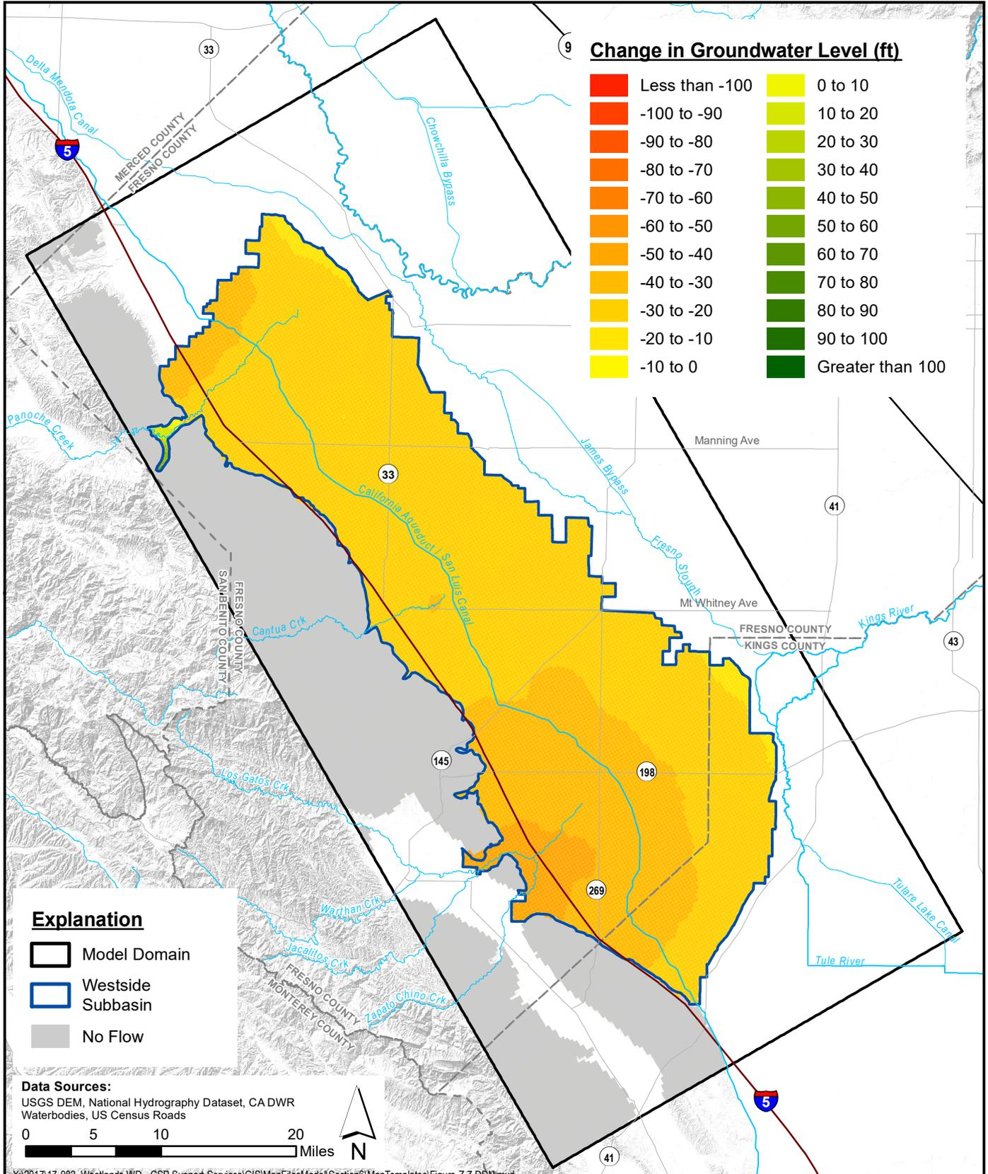
**Simulated Change in Groundwater Elevation - Lower Aquifer
