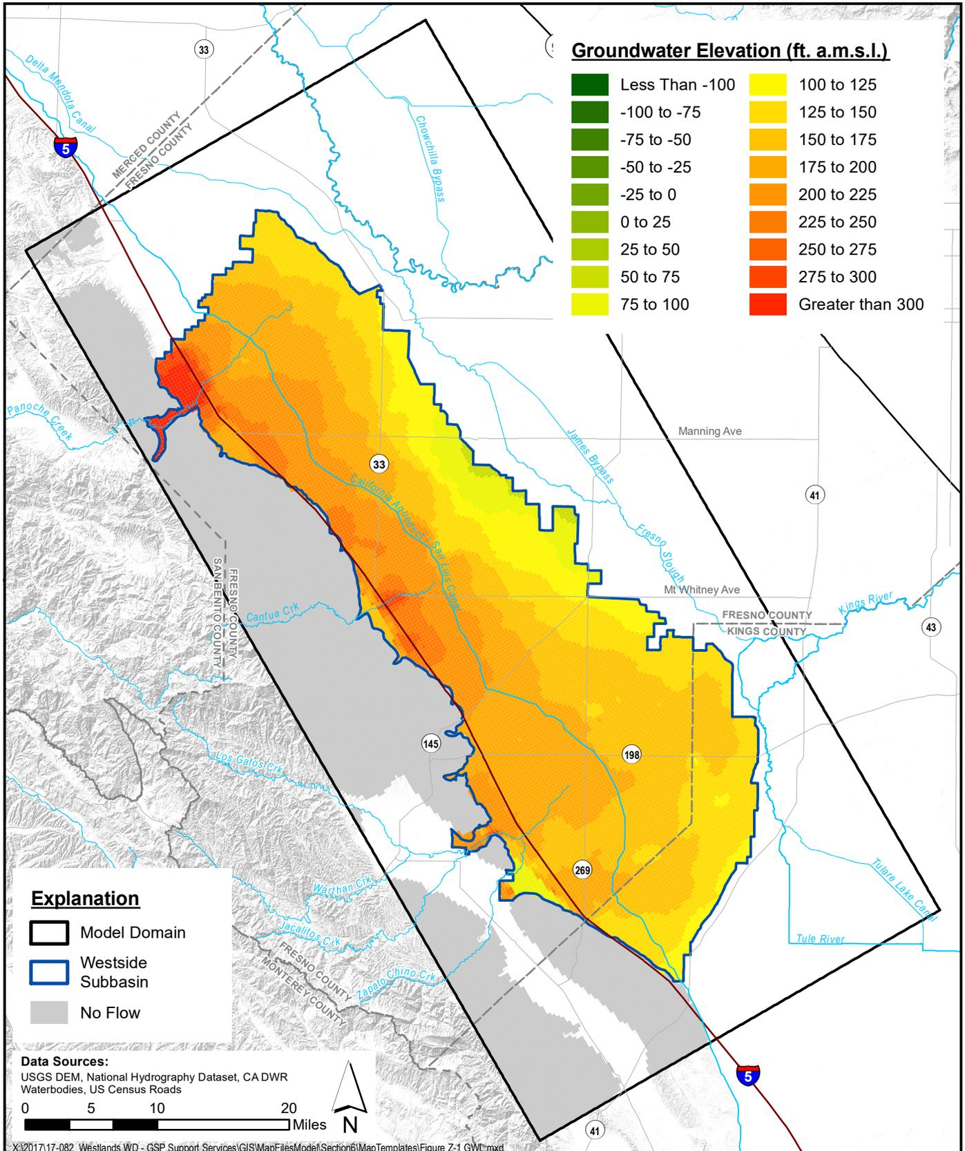
**Simulated Groundwater Elevation - Upper Aquifer
