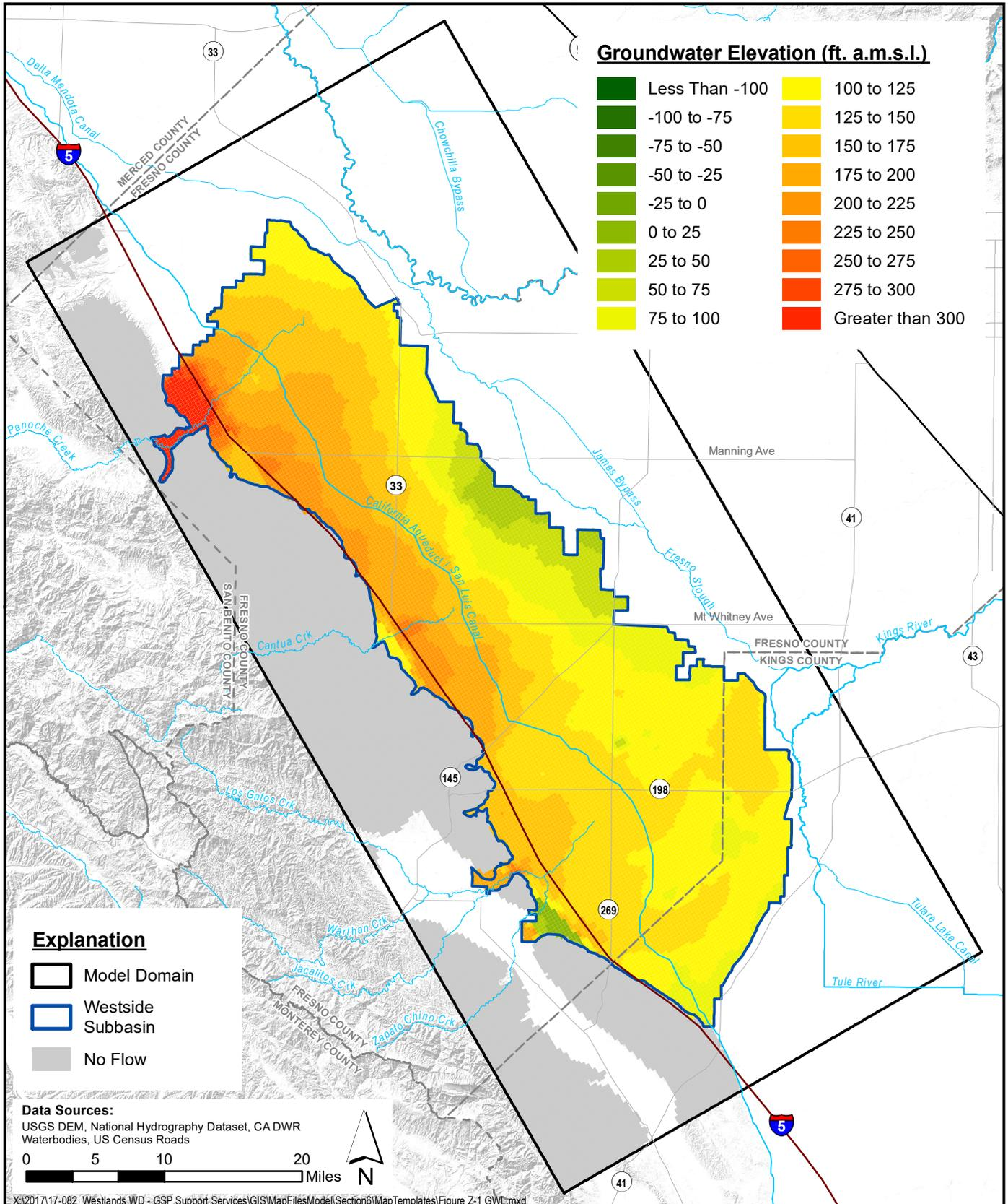
**Simulated Groundwater Elevation - Upper Aquifer
