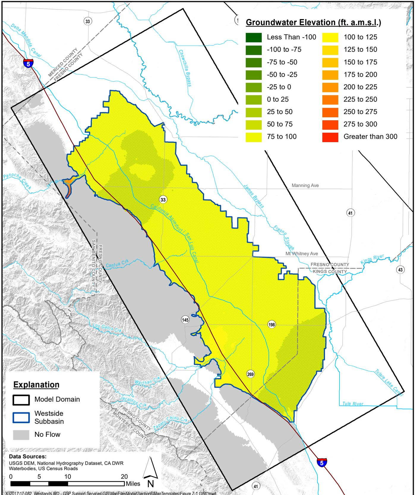
**Simulated Groundwater Elevation - Lower Aquifer
