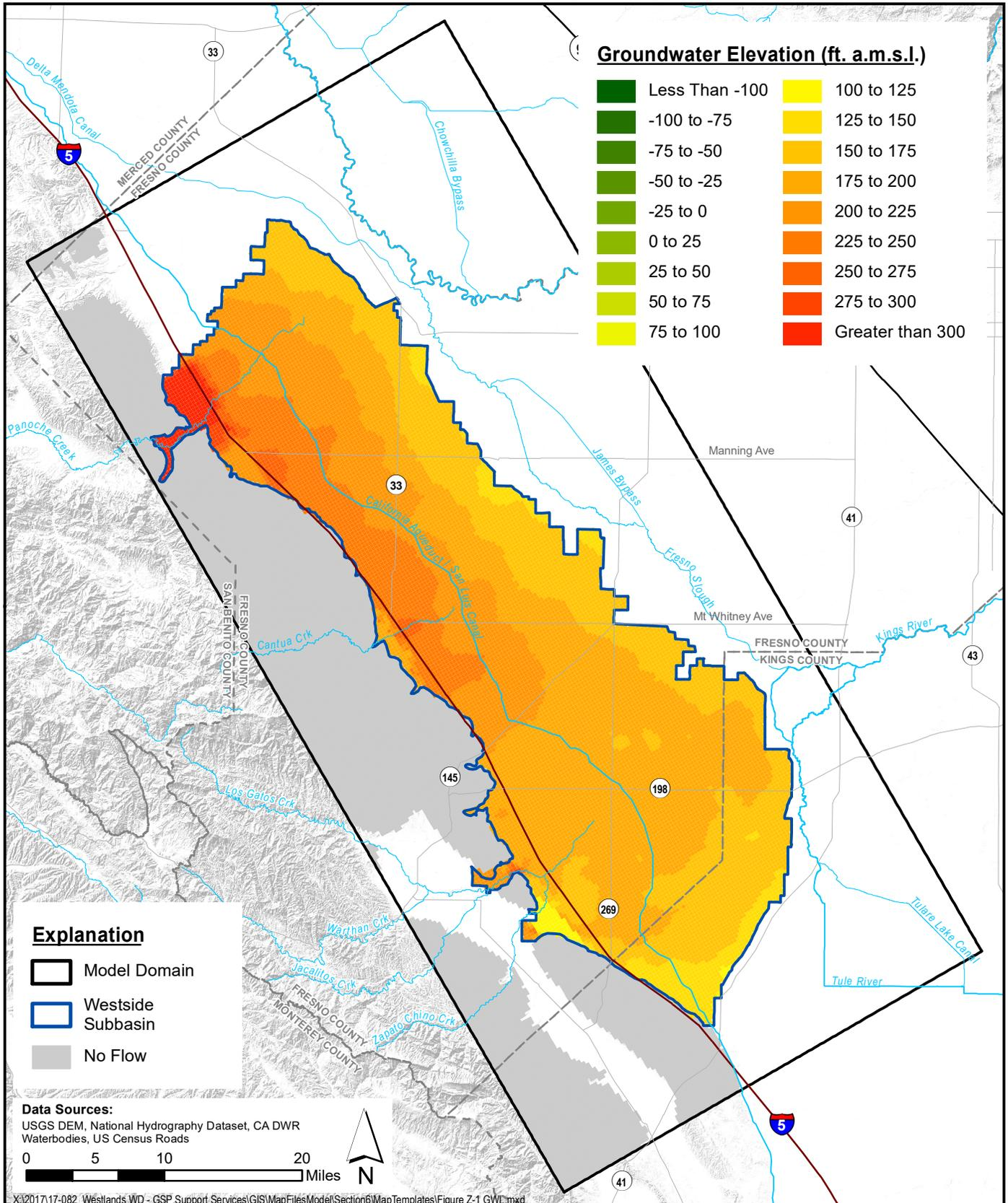
**Simulated Groundwater Elevation - Upper Aquifer
