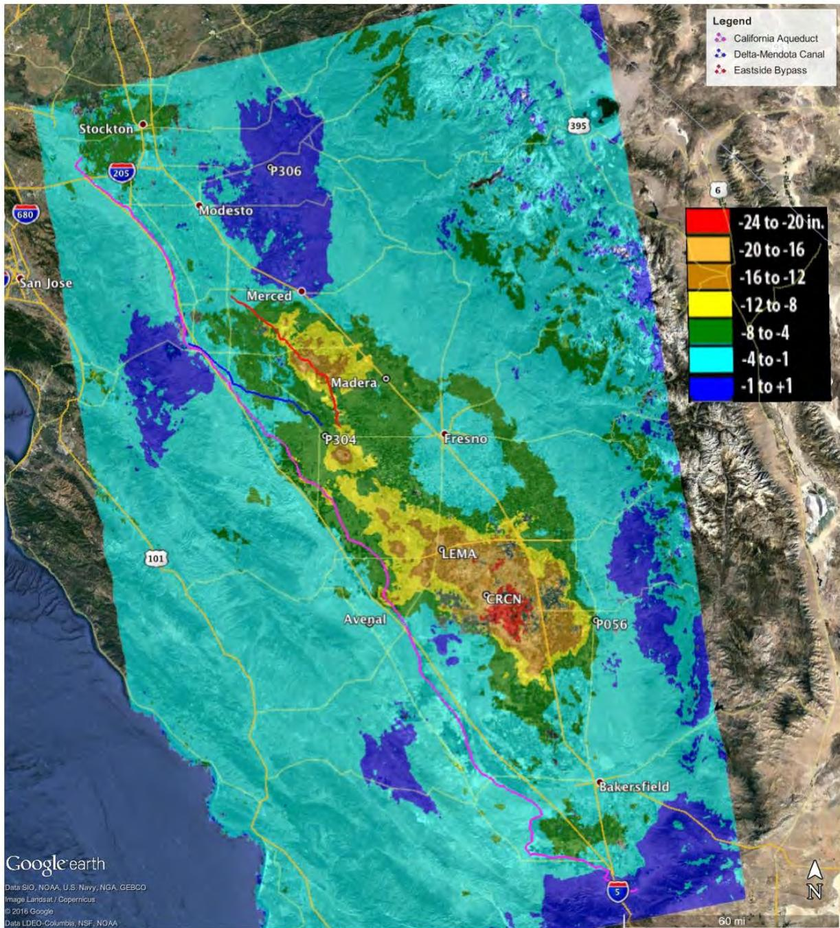
**Figure 5-116. Total Land Subsidence in San Joaquin Valley from May 7, 2015 – September 10, 2016 as measured by ESA’s Sentinel-1A and processed by JPL (Source: *Progress Report: Subsidence in California, March 2015 – September 2016*, Farr et. al. JPL, 2017)**
