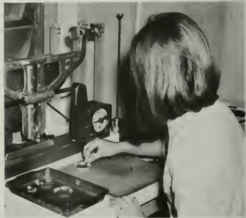
Figure 253. Determining the Plasticity Index Number of the Impervious Zone
