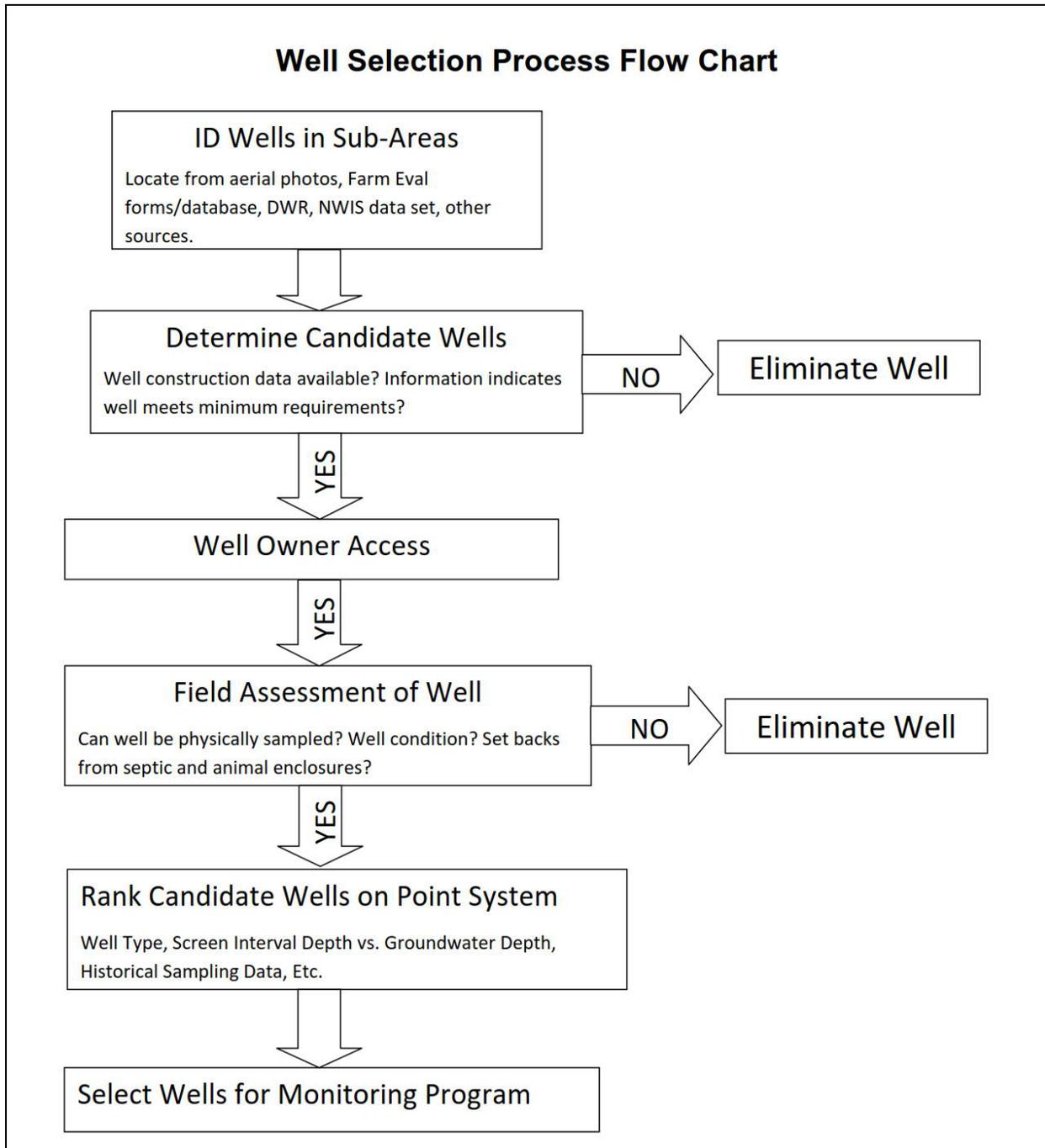
Figure 5-1. Well Selection Process Flow Chart
