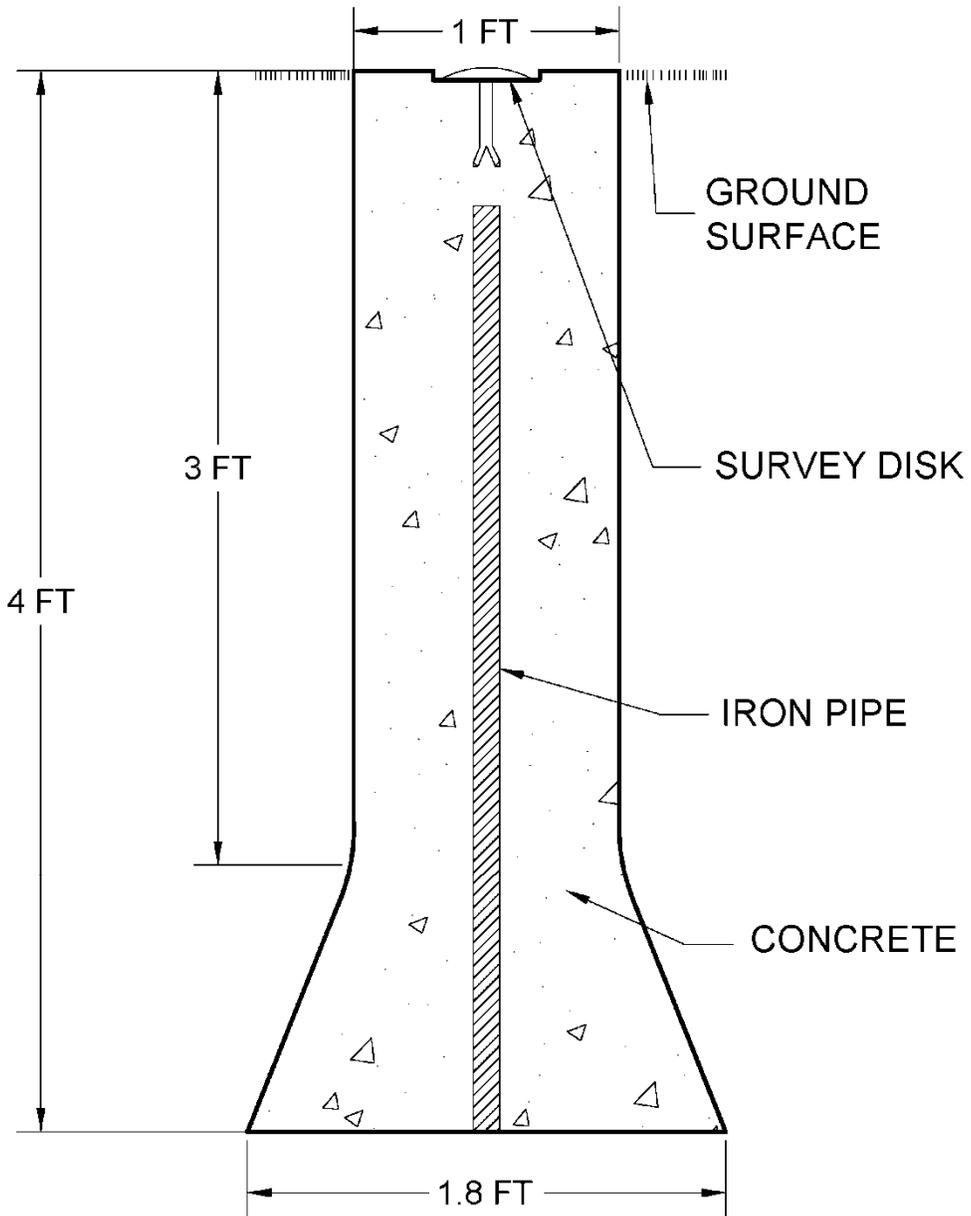
Figure 2 - Modified NGS Concrete Type Survey Monument
