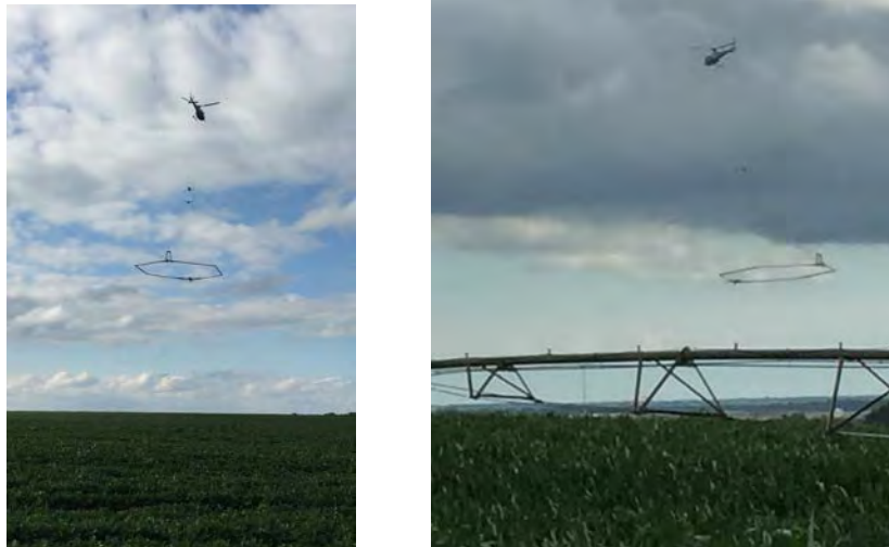
Figure 4-4: Photos of the SkyTEM312 system in suspension beneath the helicopter.
