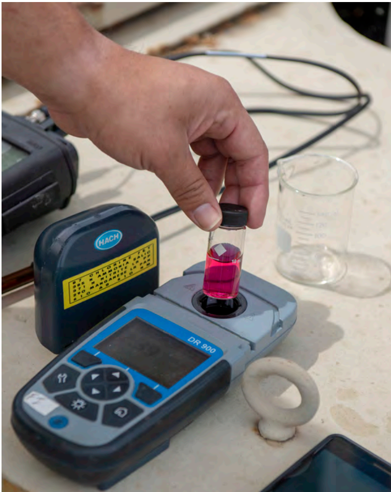
Portable instruments, such as this colorimeter, are used for testing water quality in the field.
