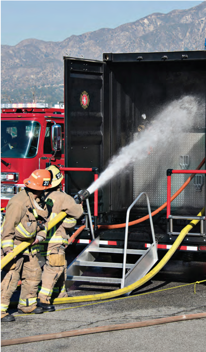
Metropolitan's Water Savings Incentive Program has paid for several fire departments (including Glendale Fire, above) to purchase equipment for firefighter training that allows water to be recirculated through pumps and fire hoses.
