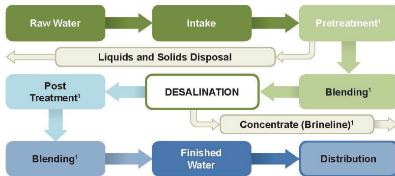
Figure 3 General Desalination System Schematic
