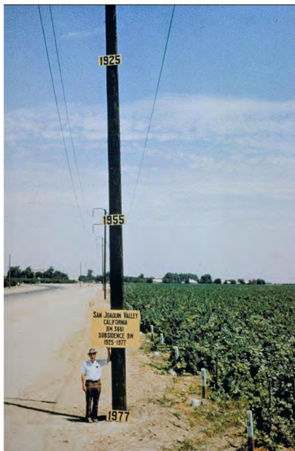
Figure 4-10. Joseph Poland standing near the location of greatest land subsidence during 1925-1977 in the San Joaquin Valley, southwest from Mendota, California. Bench mark S 661, to which subsidence at the power pole was referenced was located 31 ft southeast of the center line of Panoche Road, 2.3 ft southwest of San Joaquin Power and Light Corporation power line pole number 3/10 (replaced by a new Pacific Gas and Electric Company pole since the photograph) was not found in 1988 when NGS survey crews visited the area; it likely has been destroyed.
