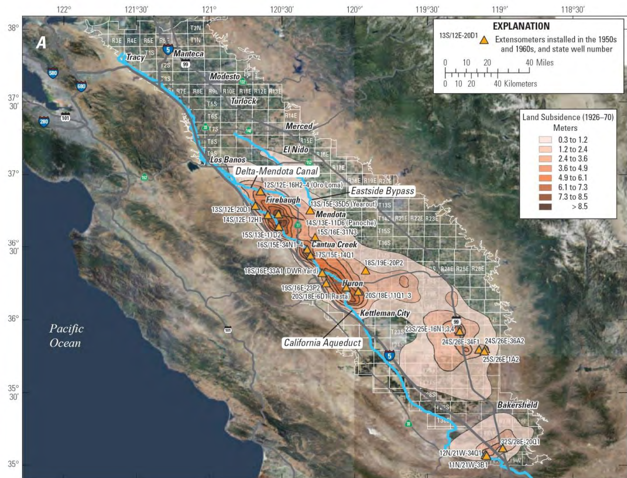
Figure 5-4. Extensometers installed in the 1950s and 1960s, San Joaquin Valley.
