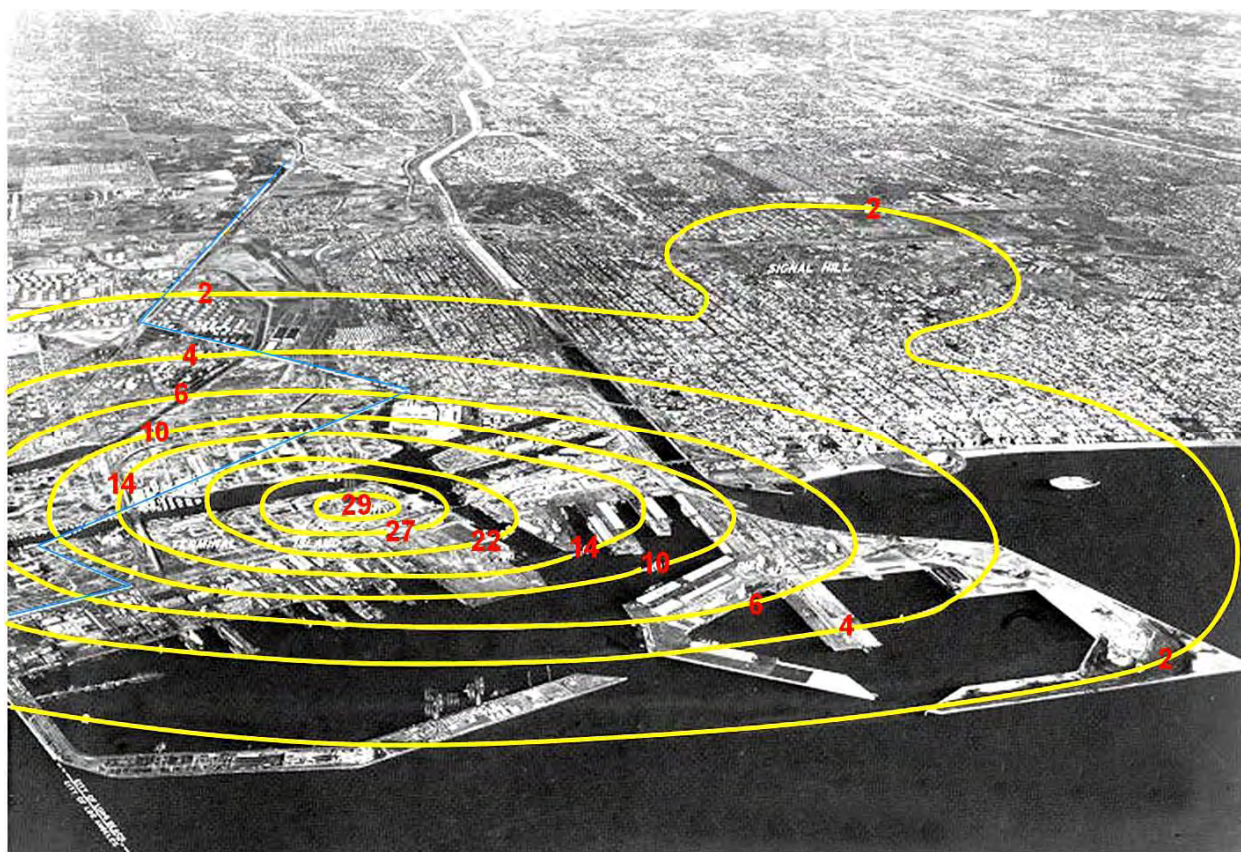
Figure A-10. Subsidence over the Wilmington Oil Field, Long Beach, California during 1928-1974, in feet (photo courtesy of John Jepson, Long Beach Gas and Oil, City of Long Beach, California).
