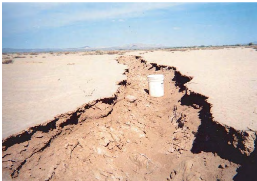
Figure 4-29. Earth fissure near the southeast edge of Lucerne Lake playa in the Mojave Desert, California. View is to the northeast, with a five-gallon bucket for scale (Sneed et al., 2003a, Fig. 6 B).
